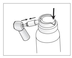
Lubrication of the chucking system
