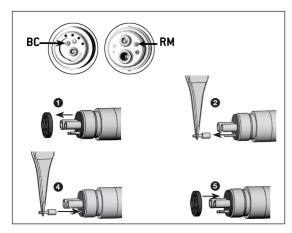
Removal/assembly of the water filter RC-98 BC/RM
