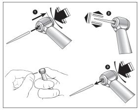
To change rotary instruments RC-95 BC/RM, RC-98 BC/RM
