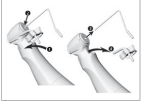
WS-75 L G, WS-75 Spray clip Coolant tube for internal bur cooling system
