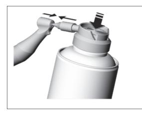
WS-91 L, WS-92 L Lubrication of the chucking system
