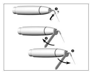
Insert/remove tip with spanner
