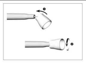
Attach the instrument changer to the instrument.
