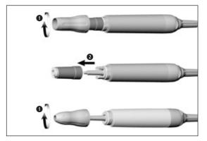
Disassembling the handpiece / Replacing of the LED socket
