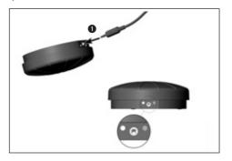
Connect the charging cable into the foot control charging socket.
