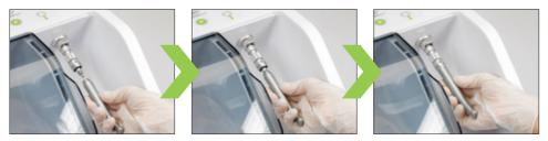
Assemble the turbine handpiece on the W&H Roto Quick adaptor
