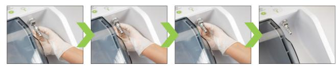
Assemble the Quick ISO adaptor on the maintenance attachment in the Assistina Twin
