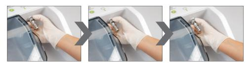
> Remove the Quick ISO adaptor from the maintenance attachment of the Assistina Twin
