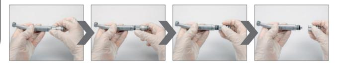
Unscrew the turbine handpiece with fix connection from the Quick RM adaptor
